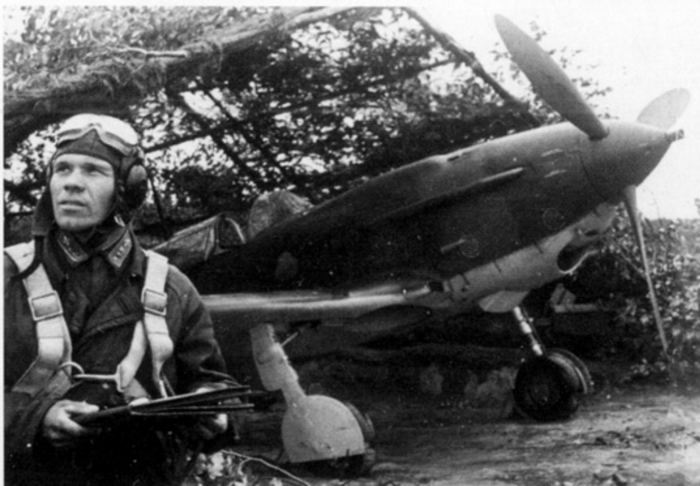
A White camouflaged early production LaGG-3 (4th Series) Red 46 being readied for a mission. The aircraft carries the insignia of a Guards Fighter Aviation Regiment above the fuselage national marking. The rudder trim tab on the rudder remained in Black Green. (Carl-Fredrik Geust)
