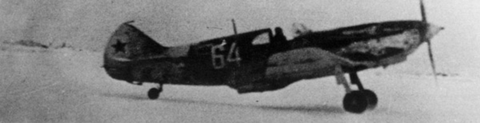
A winter camouflaged LaGG-3 (1st Series) of the 44th Fighter Aviation Regiment taxis out for a mission over the Leningrad area. The canopy and the lower main landing gear door have been removed. This LaGG-3 carries a large Red star on the rear fuselage and a small Red star on the rudder. (Robert Bock)
