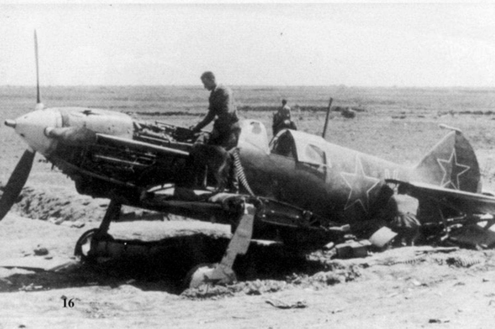
This LaGG-3 (4th Series), Red 14, was captured by Slovakian soldiers during their quick advance into the Crimea. The aircraft is unusual in that it carried White outlined national markings. (Ivo Zetik)
