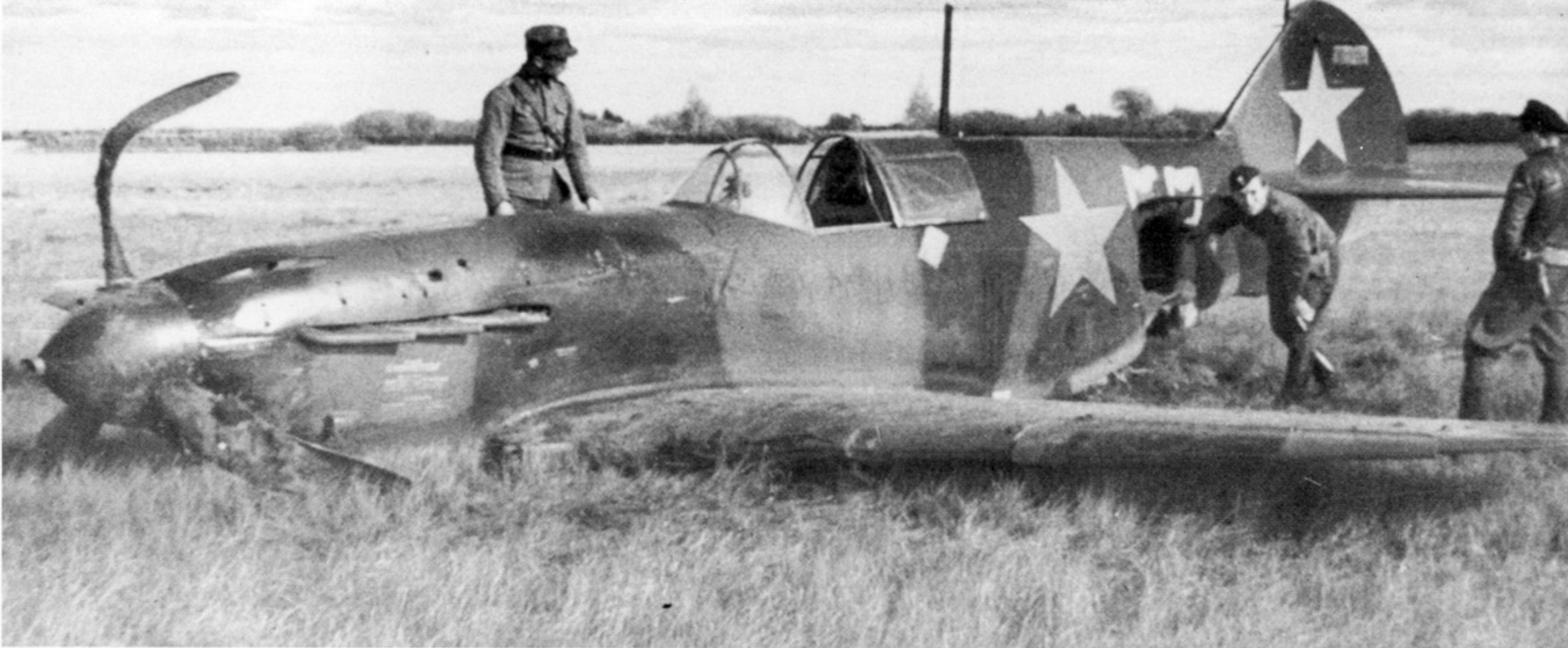
Finnish Air Force personnel look over a crash landed LaGG-3. The inspection team went over the fighter carefully to decide if it could be salvage or if it should be stripped of usable parts. In the event, the team decided that the aircraft could be put back into service. (Keski-Suomen Ilmailumuseo via Hannu Valtonen)
