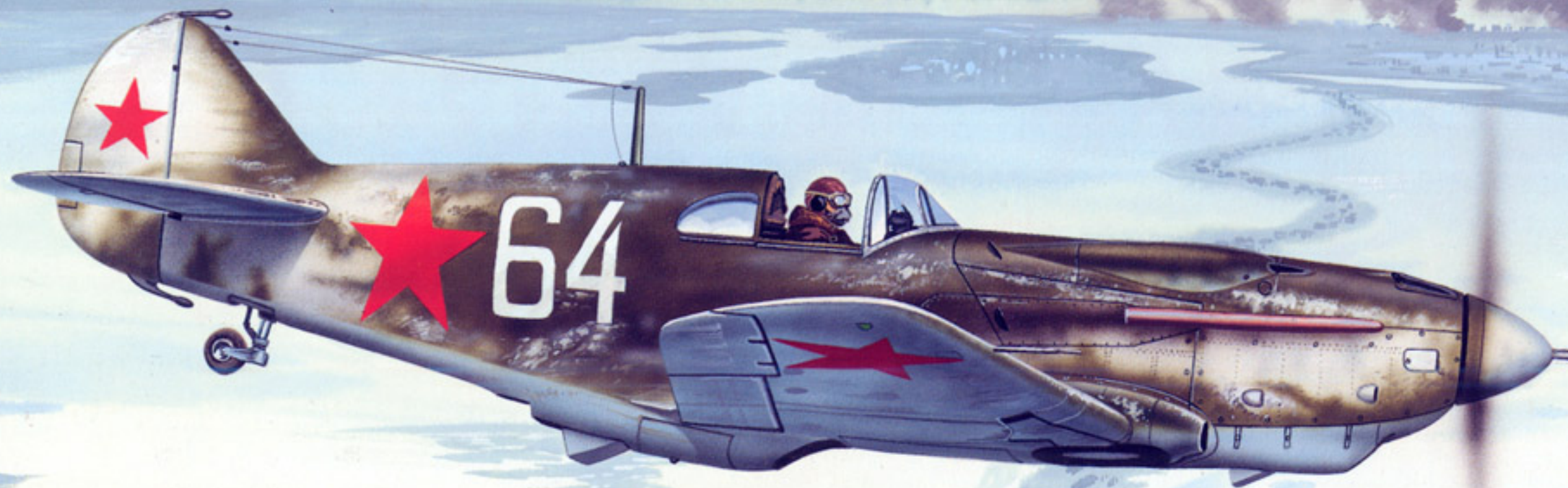
White 64, a LaGG-3 (1st Series) patrols over the "Road of Life," the Leningrad supply route across Lake Ladoga during February of 1942. The aircraft has the canopy removed, a common feature on early LaGG-3's, since the standard canopy could not be jettisoned in an emergency.
